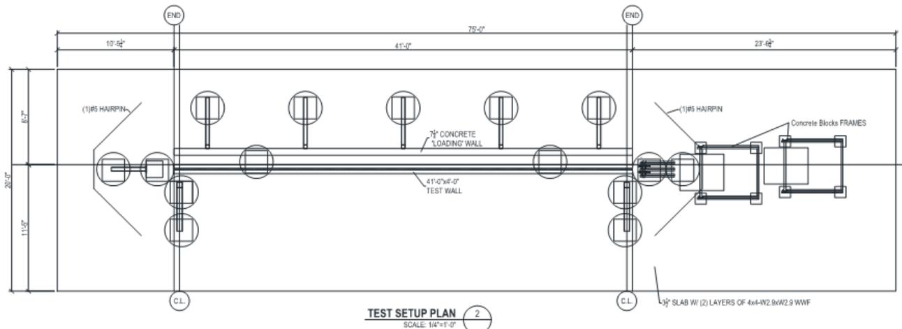
Plan view of large-scale flexural test apparatus, Report Figure 3-24, page 72.
