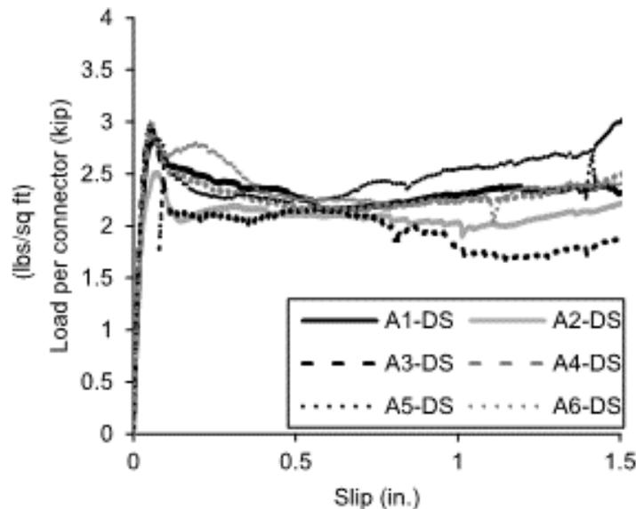
Figure 4-3a Load vs slip for double shear test (Connector A), Report page 97.
