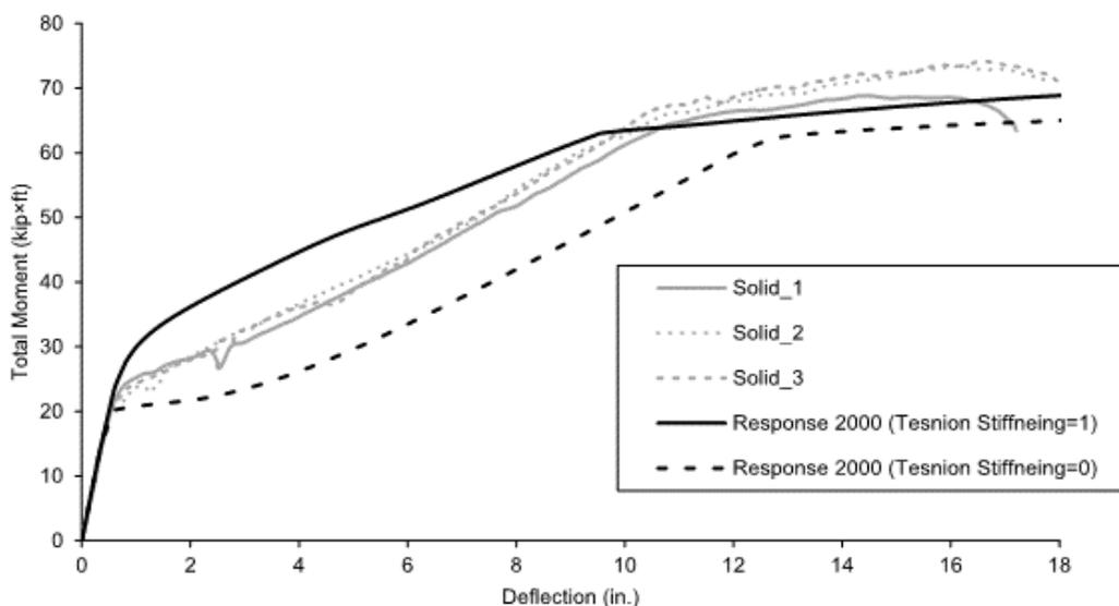
Figure 4-12: Total moment versus deflection for all solid panels, including Response 2000 with different tension stiffening rules.
